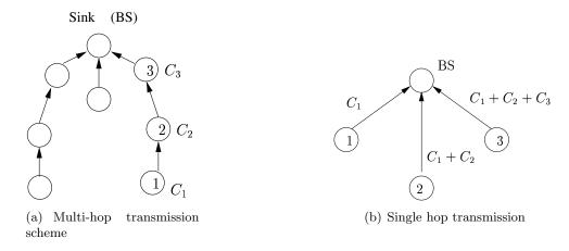
Figure 2.8: Equivalence between single hop and Multi-hop transmission.
