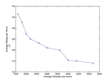
Figure 5.4: Power-Distortion curve
