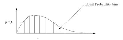
Figure 4.2: Discretization of Rayleigh channel
