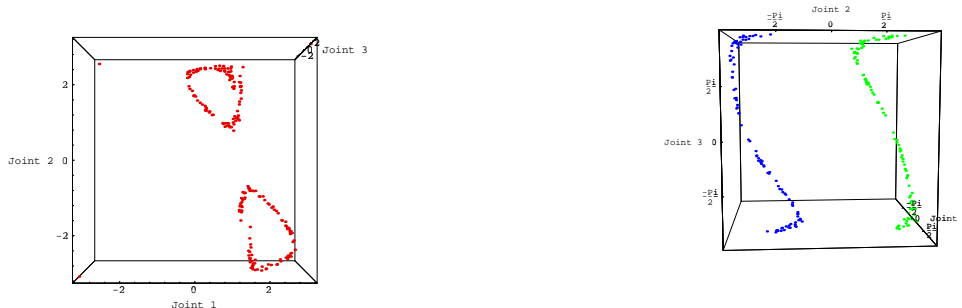
Figure 1: The two pre-image manifolds for positioning the end-effector of the 3-R planar manipulator at a specific (x, y) location.
